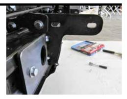
Install rear mounting bracket to front mounting bracket at top using two (2) M10 x 40 bolts, flat washers, spring washers and nuts. In lower hole of rear mounting bracket fit one M10 x 85mm bolt, flat washers and nyloc nut.
